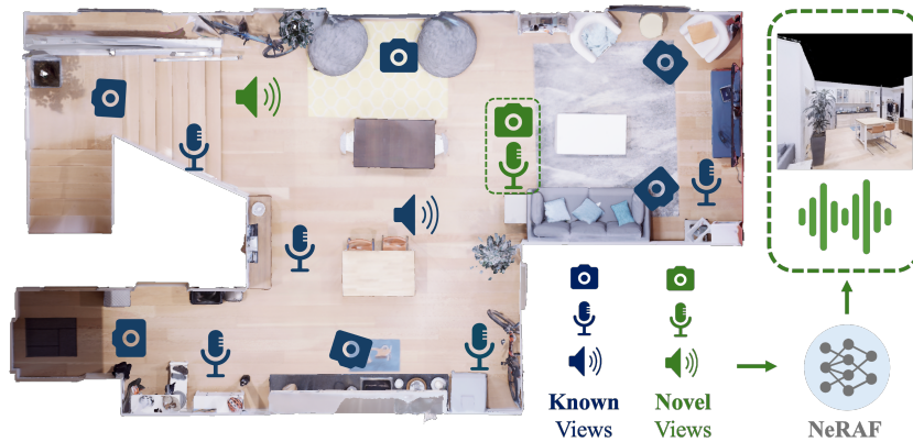
Figure 1: NeRAF synthesizes audio-visual data at novel sensor positions by learning radiance and acoustic fields from a collection of images and audio recordings. It enables audio auralization and spatialization, as well as improved image rendering, all of which are crucial for creating a realistic perception of space. NeRAF leverages cross-modal learning without the need for co-located audio and visual sensors for training. Our method allows for the independent rendering of each modality.
