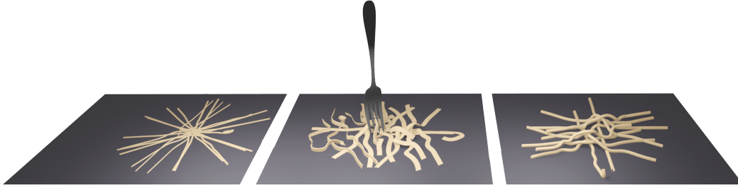
Figure 8: Blender Food Simulation Environment: We implement a custom food manipulation simulator in Blender 2.92 with an Open AI gym-style environment. The simulator supports softbody objects, such as noodles in different shape variations, as well as rigid, granular piles of items. We implement cutlery with arbitrary utensil meshes such as forks and spoons, and implement actions using the keyframing feature of Blender to control the position and orientation of a tool across frames.
