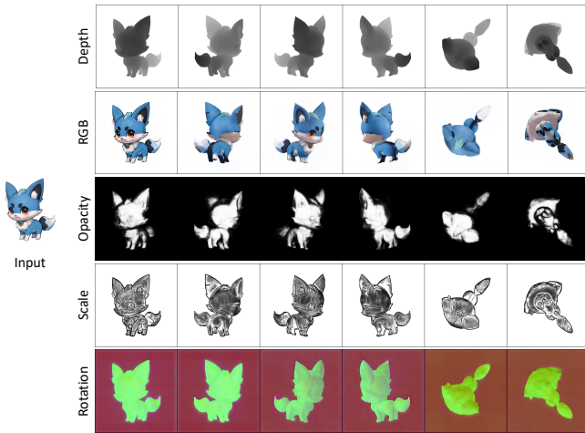
Figure 1. An example of our generated multi-view depth, RGB, and Gaussian feature images. For rotation of quaternion \mathbf{q} \in \mathbb{R}^4 , we visualize its last three channels.
