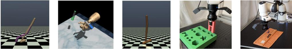
Figure 4: **Tasks in our experimental evaluation:** Benchmark tasks Walker2d, Pen, and Hopper and two vision-based contact-rich manipulation tasks on a real robot. The benchmark tasks require handling complex high-dimensional dynamics and underactuation. The robotic insertion task requires additionally addressing complex inputs such as images, non-differentiable dynamics such as contact, and all sensor noise associated with real-world robotic settings.
