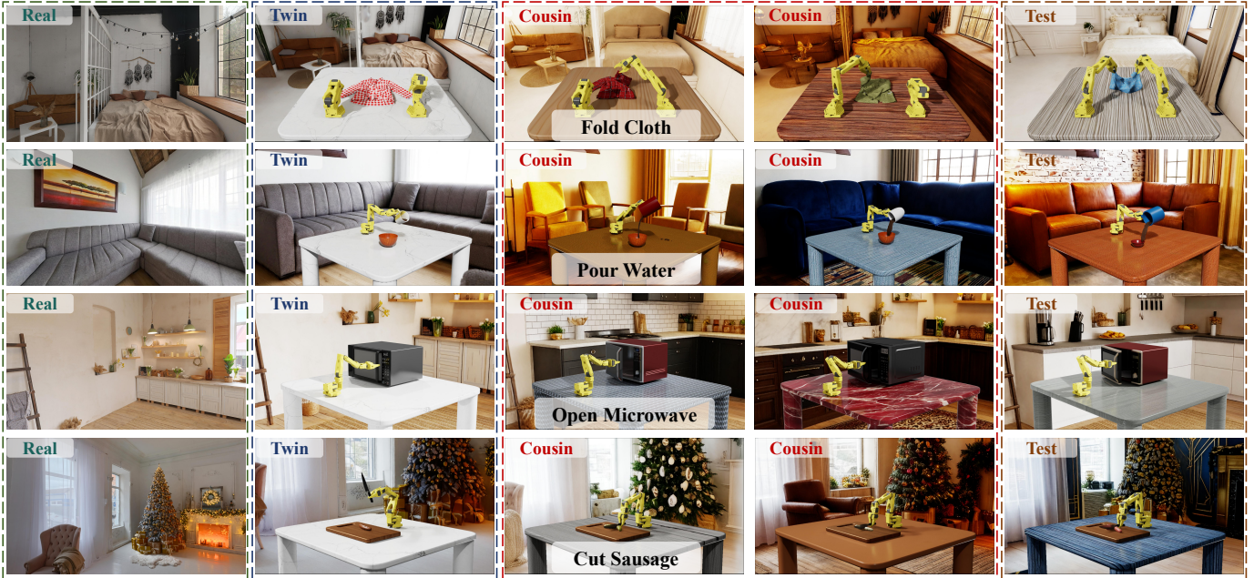
Fig. 3: Simulation Tasks and Digital Cousin Generation. Our pipeline supports a diverse range of high-fidelity simulation tasks. And each row demonstrates the transition from a sparse real-world capture ( Real ) to a precise digital reconstruction ( Twin ), followed by the generation of multiple Digital Cousins .
