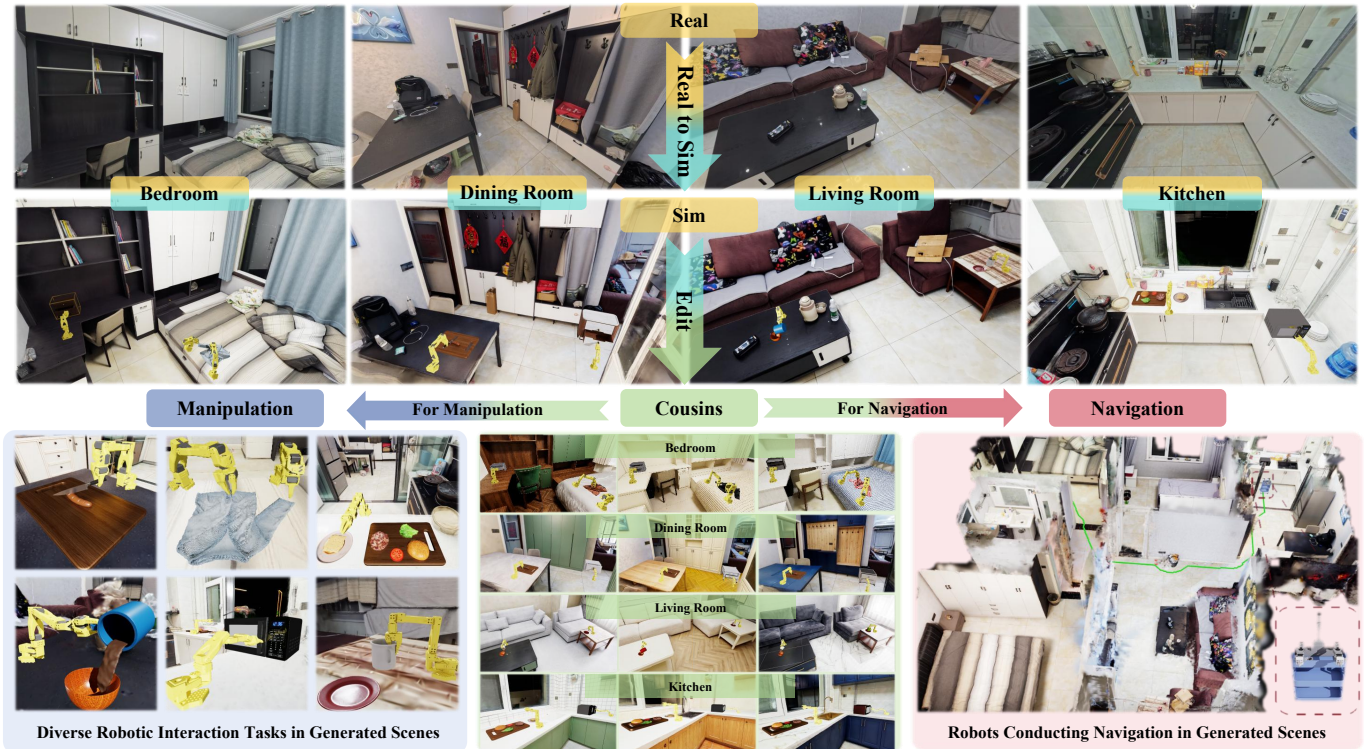
Fig. 1: WorldComposer generates high-fidelity simulation scenes from real-world panorama, and further generates diverse cousin scenes through editing. The generated rooms can be seamlessly stitched together into multi-room environments for navigation. Combined with interactive tasks, we provide a platform for generalizable learning and evaluation.
