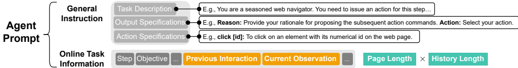
Figure 3: The components of our web navigation agent’s prompt. It includes a general instruction outlining the task, the desired output and available actions, as well as online task information providing the current goal, the agent’s past interactions, and the latest observations. Notably, the sections on previous interactions and current observation use the most tokens, and can be attributed to two main factors: the length of the pages and the extent of history span.
