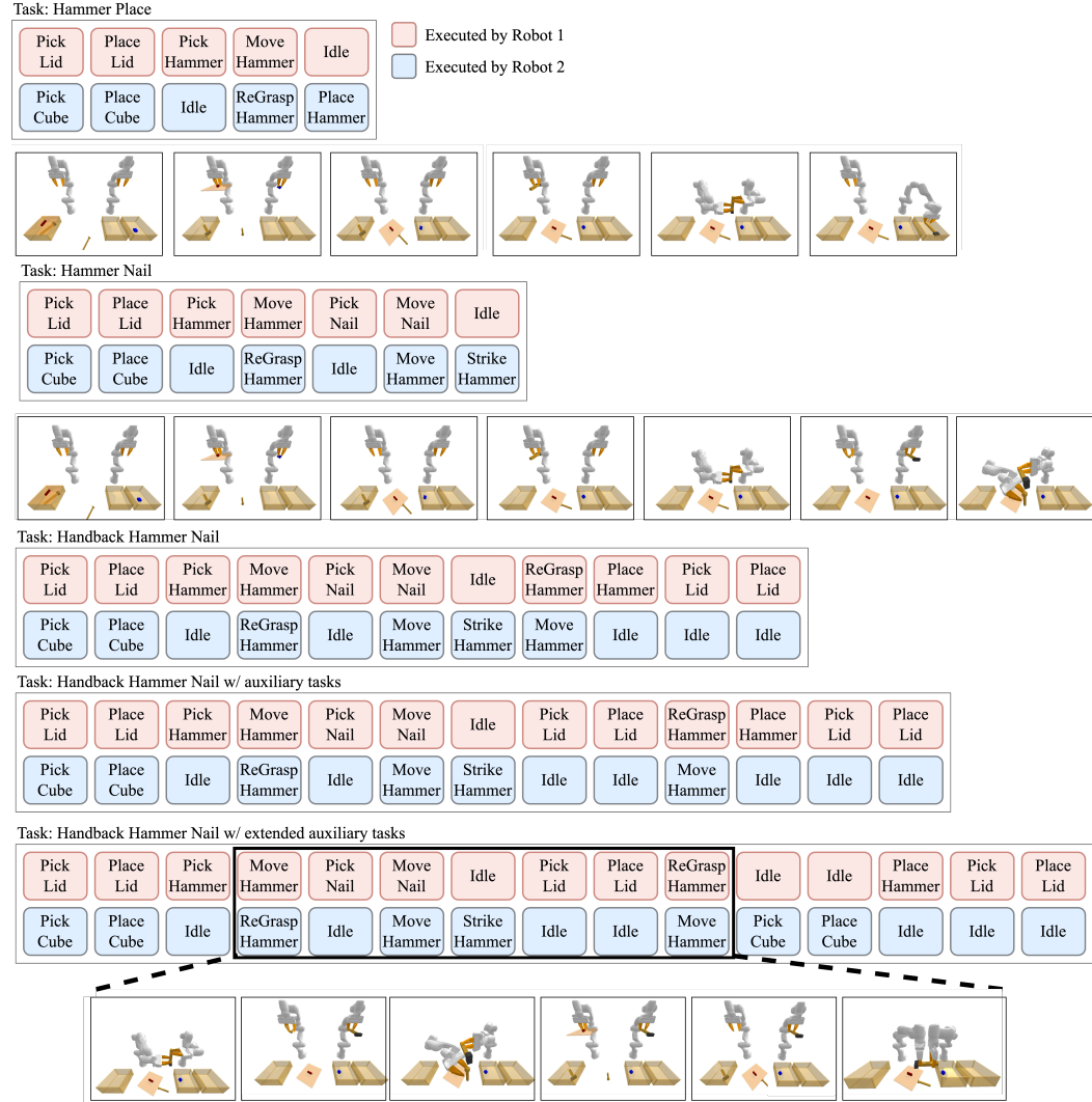
Figure S11: Extension of Hammer Nail task. We have added three new extensions to the Hammer Nail task. All of the new tasks focus on handling a second handover. The nature of the first handover adds further constraints into possible ways to perform the second handover. Further, we add task-irrelevant skills in between the plan skeleton to evaluate the robustness of GFC and the spatial-temporal factor graph plan representation.
