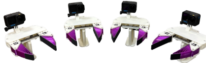
Figure 18: UMI hand-held grippers. We do not install side mirrors on the grippers.
