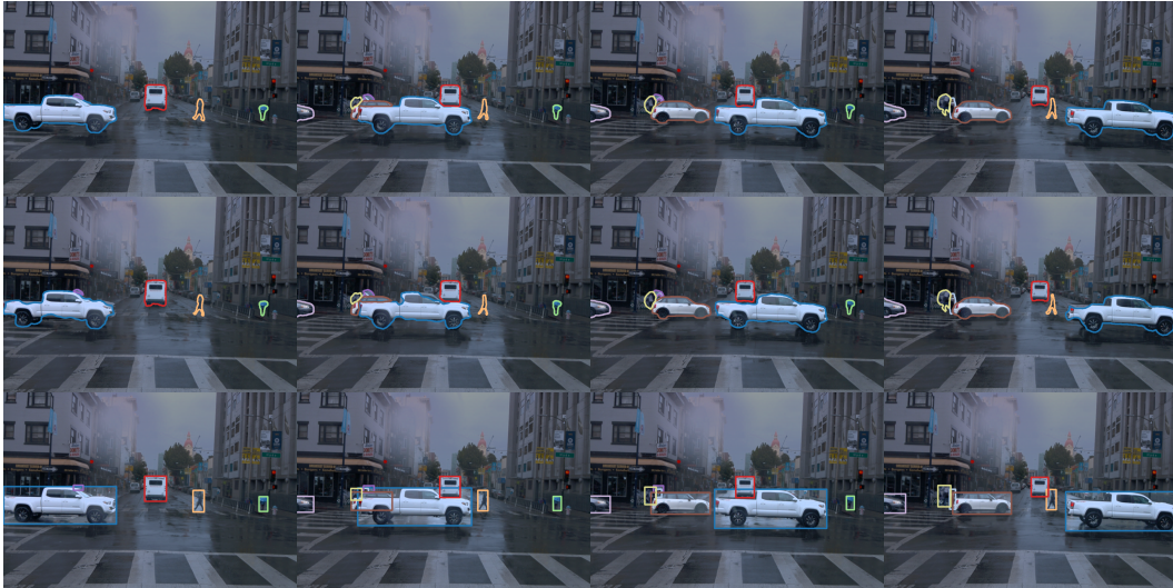
Figure 5: Ground truth references and masks (top) and their corrupted versions using morphological operations (middle) as well as axis-aligned bounding box masks (bottom). We showcase four frames of the s-141 sequence (timestamps 40, 45, 50, 55), with 0.5 seconds spacing. The morphological masks show significant aberrated and time-varying borders, while the imprecision of bounding boxes pose a challenge on addressing overlapping.
