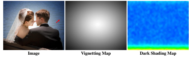
Figure 2: Coordinate-dependent distortion. The left side is the captured image, and the right side is the vignetting distribution map. The middle of the picture on the left is brighter.
