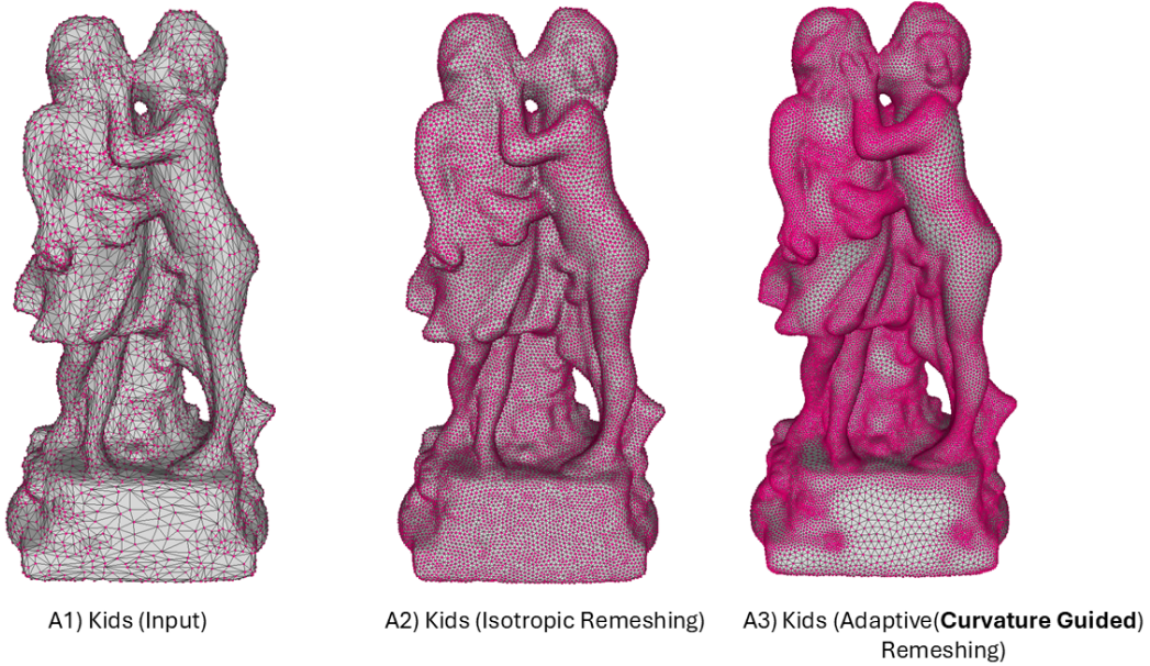
Figure 6. Qualitative comparisons between isotropic remeshing and adaptive (curvature-guided) remeshing , highlighting finer resolutions in high-curvature regions and coarser resolutions in low curvature regions.
