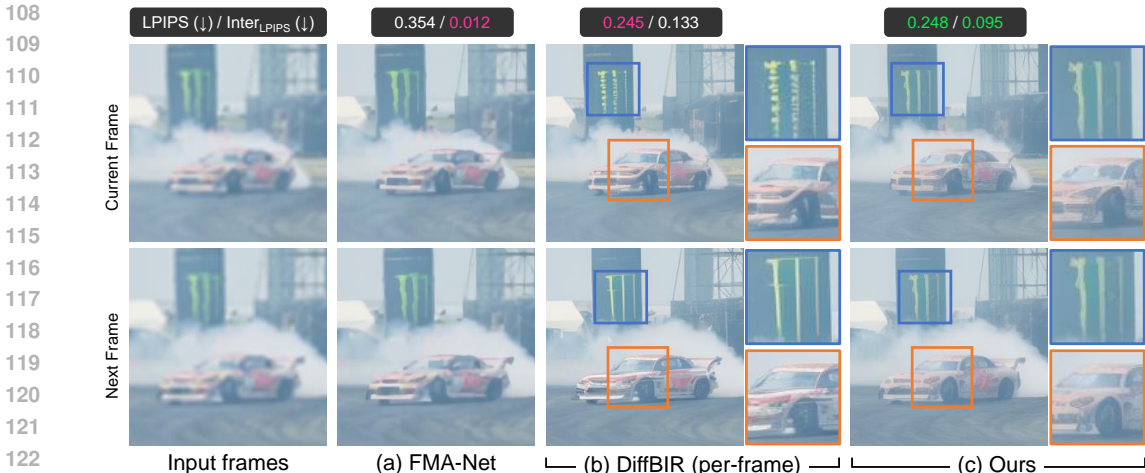
Figure 2: 4× video super-resolution results. (a) Traditional regression-based methods such as FMA-Net (Youk et al., 2024) are limited to the training data domain and tend to produce blurry results when encountering out-of-domain inputs. (b) Although applying image-based diffusion models such as DiffBIR (Lin et al., 2024) to individual frames can generate realistic details, these details often lack consistency across frames. (c) Our method leverages an image diffusion model to restore videos, achieving both realistic and consistent results without any additional training.
