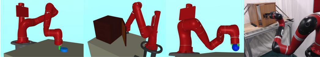
Figure 4: We evaluate on these continuous control environments. From left to right: *Visual Pusher*, a simulated pushing task; *Visual Door*, a door opening task; *Visual Pickup*, a picking task; and *Real World Visual Door*, a real world door opening task. All tasks are solved from images and without any task-specific reward. See Appendix D for details.
