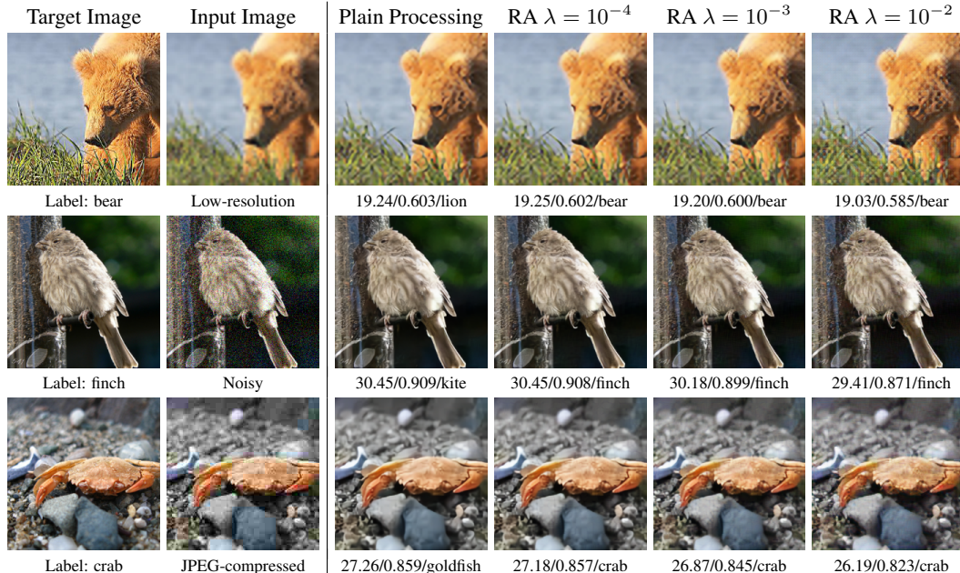
Figure 3: Examples where outputs of RA processing models can be correctly classified but those from plain processing models cannot. PSNR/SSIM/class prediction is shown below each output image. Slight differences between images from plain processing and RA processing models could be noticed when zoomed in.
