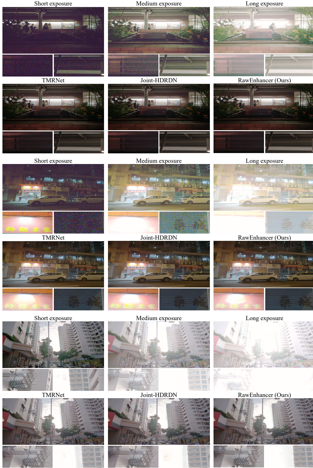
Figure 5: Visual comparison on real multi-exposure scenarios Liu et al. (2023). The reconstructed results of the listed methods exhibit noticeable artifacts, whereas our RawEnhancer consistently reconstructs images with better detail and structure across various complex exposures.
