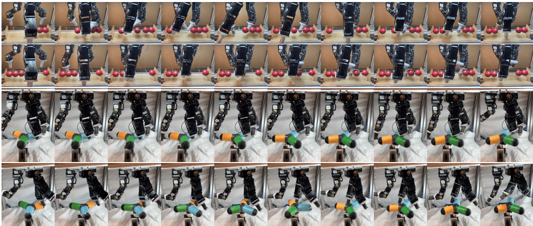
Figure 8: Evaluation rollouts of R3L on the real world tasks, for policies trained without instrumentation. The top two rows depict successful evaluation rollouts of the bead manipulation task from two distinct initial configurations. The bottom two rows depict successful rollouts of the valve rotation task. For more details on the tasks and objectives, refer to Appendix C.
