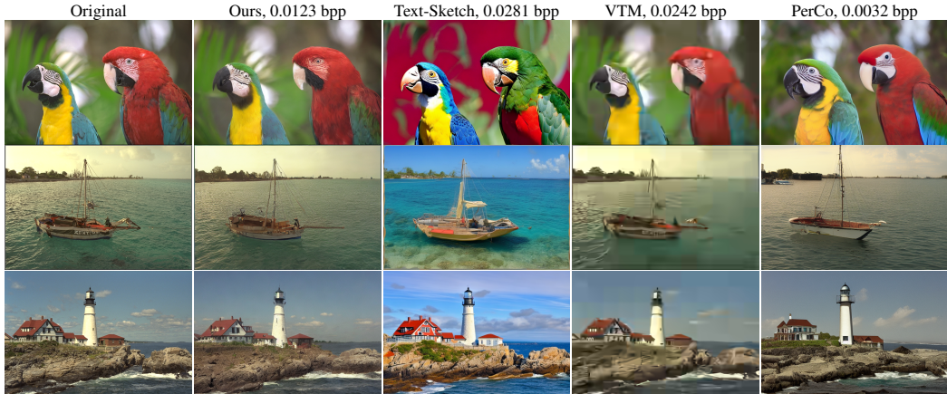
Figure 1: Kodak images compressed using our method on Stable Diffusion 1.5, Text-Sketch-PICS (Lei et al., 2023), VTM (vtm), and PerCo Careil et al. (2024). Text+Sketch/VTM/PerCo images are taken from Careil et al. (2024)
