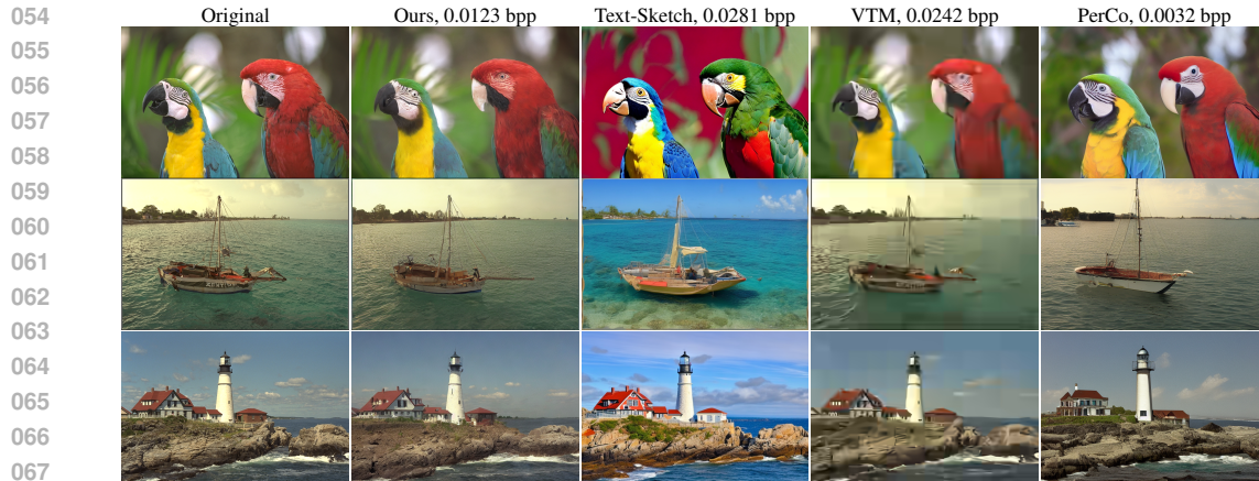
068 Figure 1: Kodak images compressed using our method on Stable Diffusion 1.5, Text-Sketch- 069 PICS (Lei et al., 2023), VTM (vtm), and PerCo Careil et al. (2024). Text+Sketch/VTM/PerCo 070 images are taken from Careil et al. (2024)
