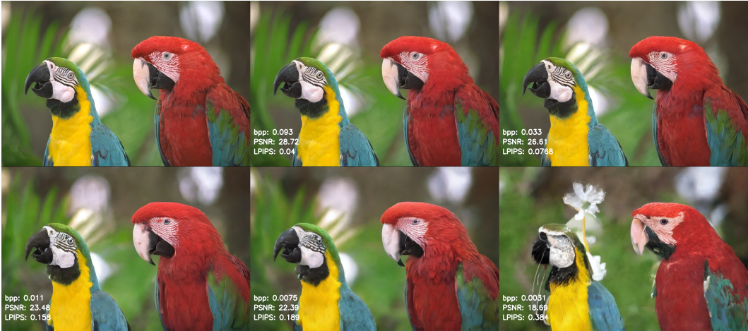
Figure 5: Reconstructions using simulated, theoretically ideal reverse-channel coding. This represents an upper bound of what results are achievable with this algorithm in principle using Stable Diffusion 1.5. Further improvements to our reverse channel coding scheme could bring actual results closer to these.
