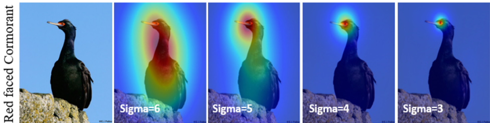
Figure 1: Salient explanation. As the value of \sigma decreases, the heat map concentrates more and more on the most discriminative part of the relevant objects, the bird’s face in this case. The salient explanation is very important for a variety of tasks such as the fine-grained classification and biomarker discovery in medical image. Note that the salient explanation is possible due to our idea of adopting Gaussian mask.
