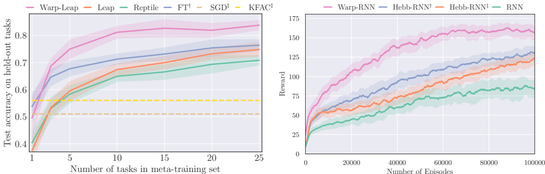
Figure 4: Left : Omniglot test accuracies on held-out tasks after meta-training on a varying number of tasks. Shading represents standard deviation across 10 independent runs. We compare Warp-Leap, Leap, and Reptile, multi-headed finetuning, as well as SGD and KFAC which used random initialisation but with 10x larger batch size and learning rate. Right : On a RL maze navigation task, mean cumulative return is shown. Shading represents inter-quartile ranges across 10 independent runs. †Simple modulation and ‡retroactive modulation are used (Miconi et al., 2019).
