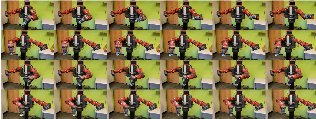
Figure 7: Depiction of execution of additional learned primitives on real world Baxter robot. As in Fig. 4, each row is a single primitive, while columns show progress of the primitive over time. Row 1 depicts a left handed returning primitive, row 2 depicts a right handed pushing primitive, row 3 depicts a left handed pushing primitive (in a different configuration to the left handed one), and finally row 4 depicts a right handed twisting primitive.
