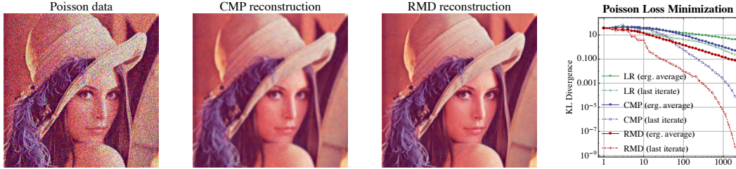
Figure 1: Reconstruction of the Lena test image from a sample contaminated with Poisson noise. Left to right: (a) the contaminated sample; (b) CMP reconstruction; (c) RMD reconstruction; and (d) Poisson likelihood loss at each iteration. The RMD process provides a sharper definition of image features relative to the CMP algorithm (which is the second-best); higher-definition images and more details can be found in the appendix.
