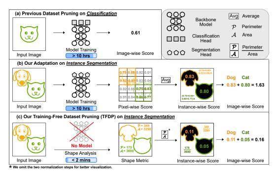
Figure 3: Comparison of different dataset pruning pipelines. (a) Pruning classification dataset requires model training. (b) Our adaptation of previous methods on instance segmentation by training a segemntation head and computing the importance score for each pixel. (c) The proposed method that is training-free and model-independent.
