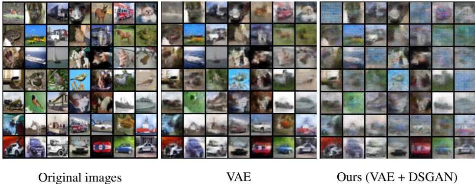
Figure 8: Comparison of the reconstructed results of the VAE and our method. The seen class, which is at the bottom of the images, is a car. Other rows are images from the unseen classes. Our method exhibits a relatively larger gap, in terms of the reconstruction error between the seen data and unseen data, than the VAE.
