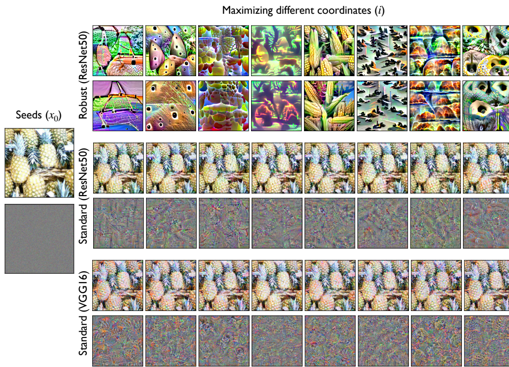
Figure 16: Correspondence between image-level patterns and activations learned by standard and robust models on the complete ImageNet dataset. Starting from randomly chosen seed inputs (noise/images), we use PGD to find inputs that (locally) maximally activate a given component of the representation vector (cf. Appendix A.6.1 for details). In the left column we have the original inputs (selected randomly ), and in subsequent columns we visualize the result of the optimization (5) for different activations, with each row starting from the same (far left) input for ( top ): a robust (adversarially trained) ResNet-50 model, ( middle ): a standard ResNet-50 model and ( bottom ): a standard VGG16 model.
