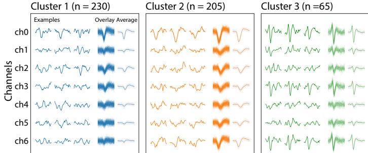
Figure 11: Synthetic data examples. Example of 500 synthetic spikes from 3 clusters.
