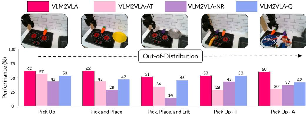
Figure 8: Comparative evaluation of VLM2VLA ablations on in-distribution (ID) and out-of-distribution (OOD) robotic manipulation tasks. VLM2VLA maintains high success rates on OOD tasks relative to ablated variants, highlighting the importance of reasoning and the robustness of our methodology across different model architectures. Each bar corresponds to an average over thirty trials, except for the ‘Pick Up - T’ task, where each bar corresponds to an average over ninety trials.
