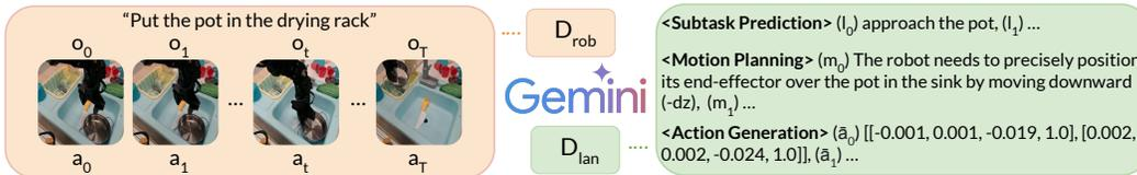
Figure 4: VLM2VLA’s pipeline for annotating existing robot datasets  $D_{rob}$  into  $D_{lan}$  described via natural language. We use Gemini 2.5 (Team, 2025) to decompose each trajectory into sub-trajectories, each with an associated subtask, motion plan, and action chunk.
