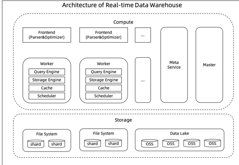
Figure 7: Architecture of the real-time data warehouse.
