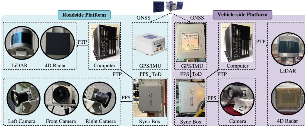
Figure 8: **The time synchronization solution for the connected vehicle-side platform and the intelligent roadside unit.** Both the vehicle platform and roadside unit are equipped with a computer, a time synchronization box, a GPS/IMU system, and various sensors, including LiDAR, 4D Radar, and cameras. The GPS/IMU systems in both the vehicle platform and roadside unit receive the same GNSS signals from GPS satellites.
