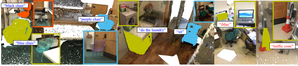
Figure-R 1: Qualitative results of UniSeg3D on the ScanNet200 dataset. We show open-vocabulary segmentation results using open-set text prompts. Red prompts mean categories that are not present in the ScanNet200 labels, while blue prompts describe the attributes of various objects, such as affordances and color. For each scene, we show the instance with the highest similarity score to the query embedding. These results highlight the model’s open-vocabulary capability.
