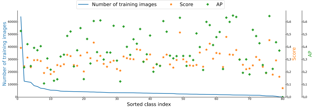
Figure A: Per-class AP of Faster R-CNN and the category distribution on MSCOCO (2017) . The categories are sorted in descending numbers of training images . Orange stars indicate the average of predicted confidence scores for each class. Green diamonds are per-class APs. The least frequent class, “hair driver”, still has 189 training images, indicating that all the classes in MSCOCO are considered as frequent classes using the definition of LVIS.
