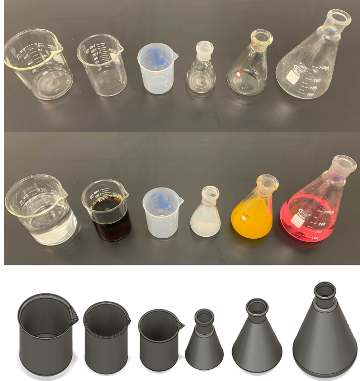
Figure 9: Six objects and corresponding 3D models used in TODD , from left to right is Beaker 1, Beaker 2, Beaker 3, Flask 1, Flask 2 and Flask 3. From top to bottom is empty objects, objects filled with five different liquids and 3D models.
