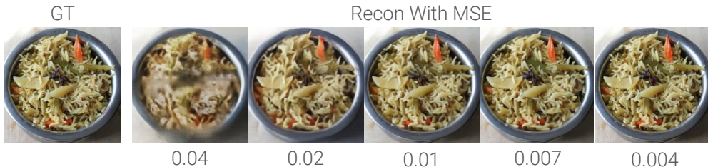
Figure 10 Comparison of reconstructed image quality at varying MSE thresholds. The ground truth (GT) image is displayed on the left, followed by reconstructions at different MSE thresholds (0.04, 0.02, 0.01, 0.007, and 0.004), showing progressive improvement in fidelity as the threshold decreases.
