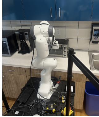
Figure 6: Real robot setup. Our real world setup features a Panda robot arm in a real world kitchen.
