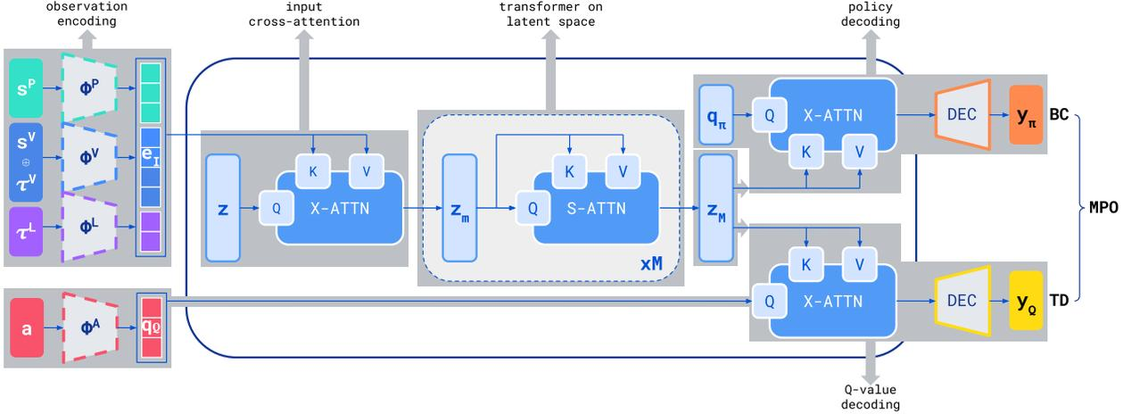
Figure 5. High-level PAC model architecture, with each sub-procedure outlined in Algorithm 1 visually grouped; note that  $z_m$  is used in both policy decoding and Q-value decoding. Details are discussed in Section B.
