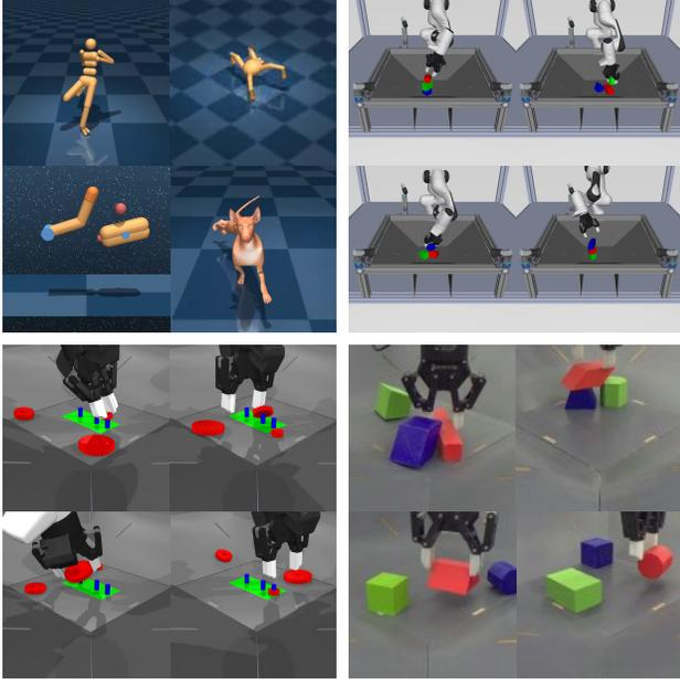
Figure 6. A selection of the domains and tasks in our data mix. **Top left:** Control Suite features 32 different continuous control tasks across 15 different embodiments with a great variance in proprioception and action spaces. **Top right:** Stacking RGB objects into different configurations (pyramides and towers) with a simulated Panda arm. **Bottom left:** Inserting gears onto pegs in simulation. **Bottom right:** Performing the RGB stacking task on a real Sawyer robot.
