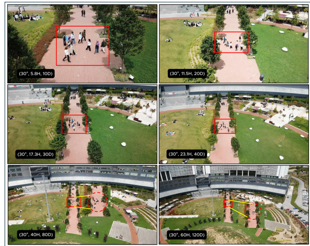
Figure 1. Illustration of extreme far-distance conditions in the DetReIDX dataset. As UAV altitude and horizontal distance increase, pedestrians undergo severe scale compression and resolution degradation. The red bounding boxes highlight the same group of individuals as their pixel footprint shrinks dramatically, showing the visual challenges of aerial-ground video person ReID.
