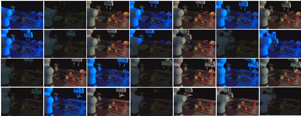
Figure 34: Light distraction. Stable visual features from DINO and SigLIP enable the model to operate robustly under extreme out-of-distribution lighting conditions.
