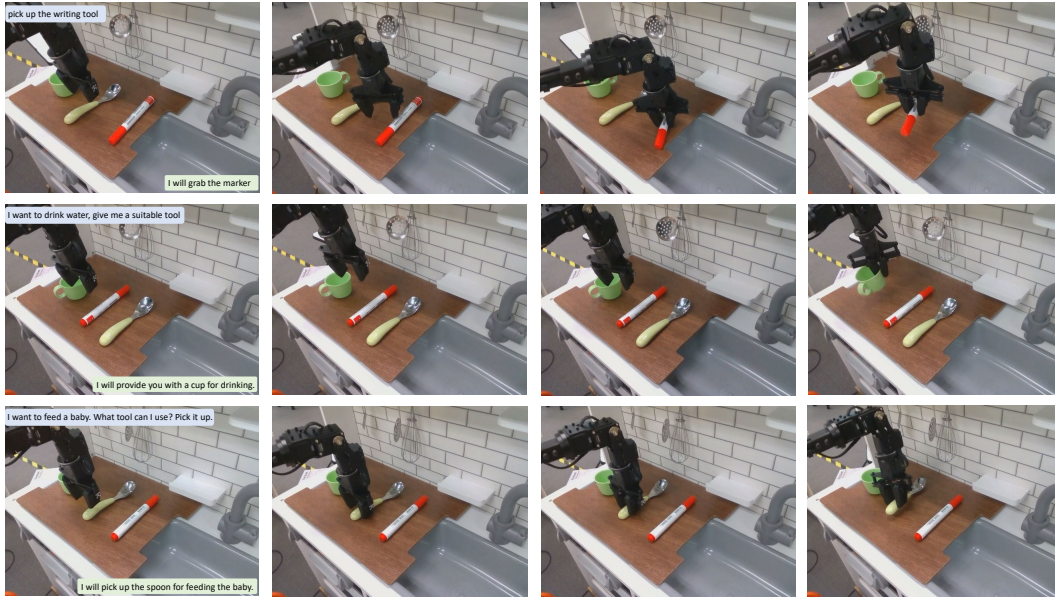
Figure 35: Zero-shot evaluation. We perform zero-shot evaluation in the Bridge kitchen environment with augmented background and novel objects. The instruction and model response are visualized in the first image.
