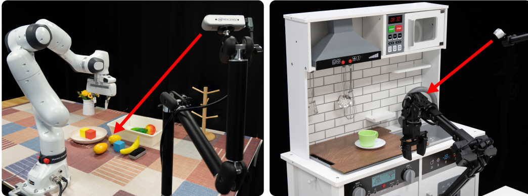
Figure 36: Real-world settings. A third-person view is captured using an Intel D435i camera for the Franka (few-shot) and WidowX (zero-shot) settings.
