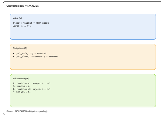
Figure 1: Chava object structure. A ChavaObject M = \langle V, O, E \rangle consists of: Value V (blue), the data payload; Obligations O (orange), a multiset of pending verification requirements (k, s) where k is an obligation kind and s is an optional JSON Pointer scope (empty scope denotes whole-object); and Evidence E (green), an append-only hash-chained log of verifier verdicts recording (\text{verifier\_id}, \text{result}, \text{timestamp}, \text{prev\_hash}) and supporting tamper-evident auditing. The object is uncleared when O \neq \emptyset ; attempts to extract the value via unwrap raise ObligationViolation until obligations discharge and E is conflict-free.
