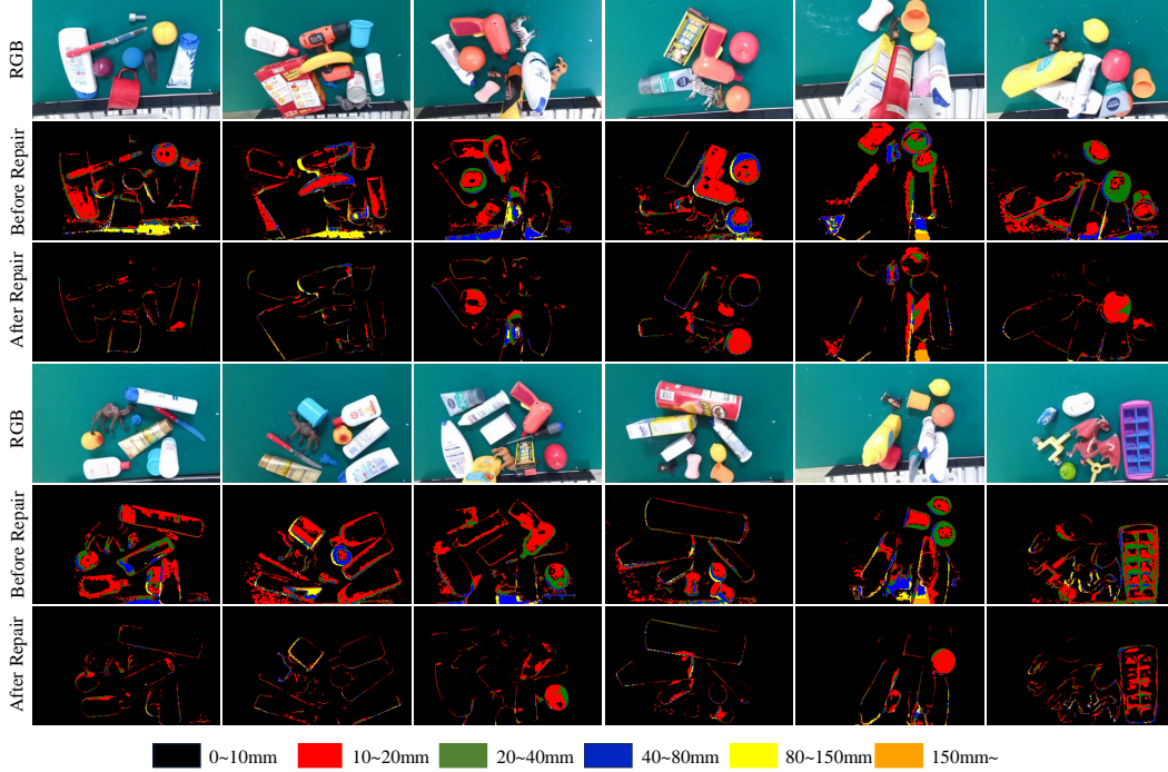
Figure S1: Comparison of camera noise before and after R2SRepairer. Different colors in the noise map represent different noise amplitude ranges, with amplitude measured in millimeters
