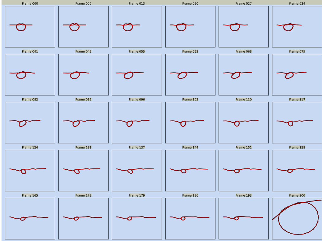
Figure 9: Illustration of the temporal evolution of a knot scenario. The rod is fixed at both ends and the knot is pulled tight. The predicted results by end-to-end COPINGNet-based learning are shown in red while the results computed with COPINGNet-assisted PBD are shown in black. The visualization of the last frame contains a close-up to demonstrate that the knot structure is still preserved.
