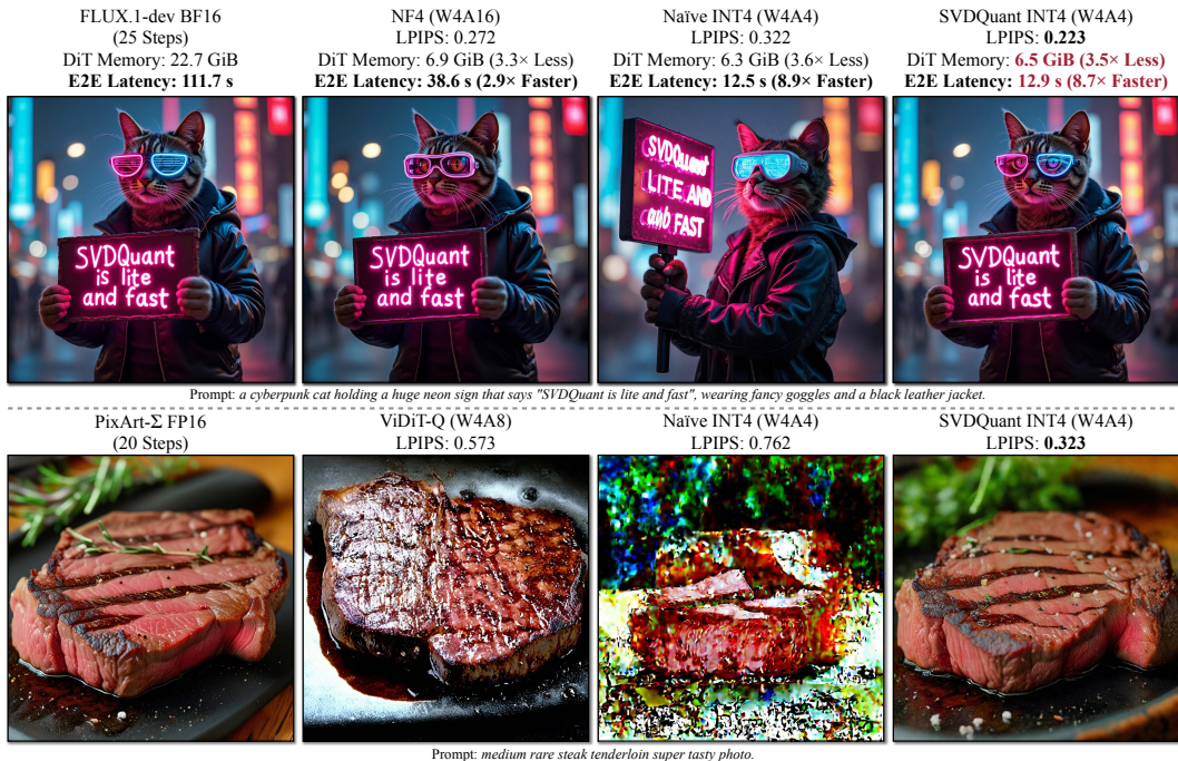
Figure 1: SVDQuant is a post-training quantization technique for 4-bit weights and activations that well maintains visual fidelity. On 12B FLUX.1-dev, it achieves 3.6× memory reduction compared to the BF16 model. By eliminating CPU offloading, it offers 8.7× speedup over the 16-bit model when on a 16GB laptop 4090 GPU, 3× faster than the NF4 W4A16 baseline. On PixArt-Σ, it demonstrates significantly superior visual quality over other W4A4 or even W4A8 baselines. “E2E” means the end-to-end latency including the text encoder and VAE decoder.
