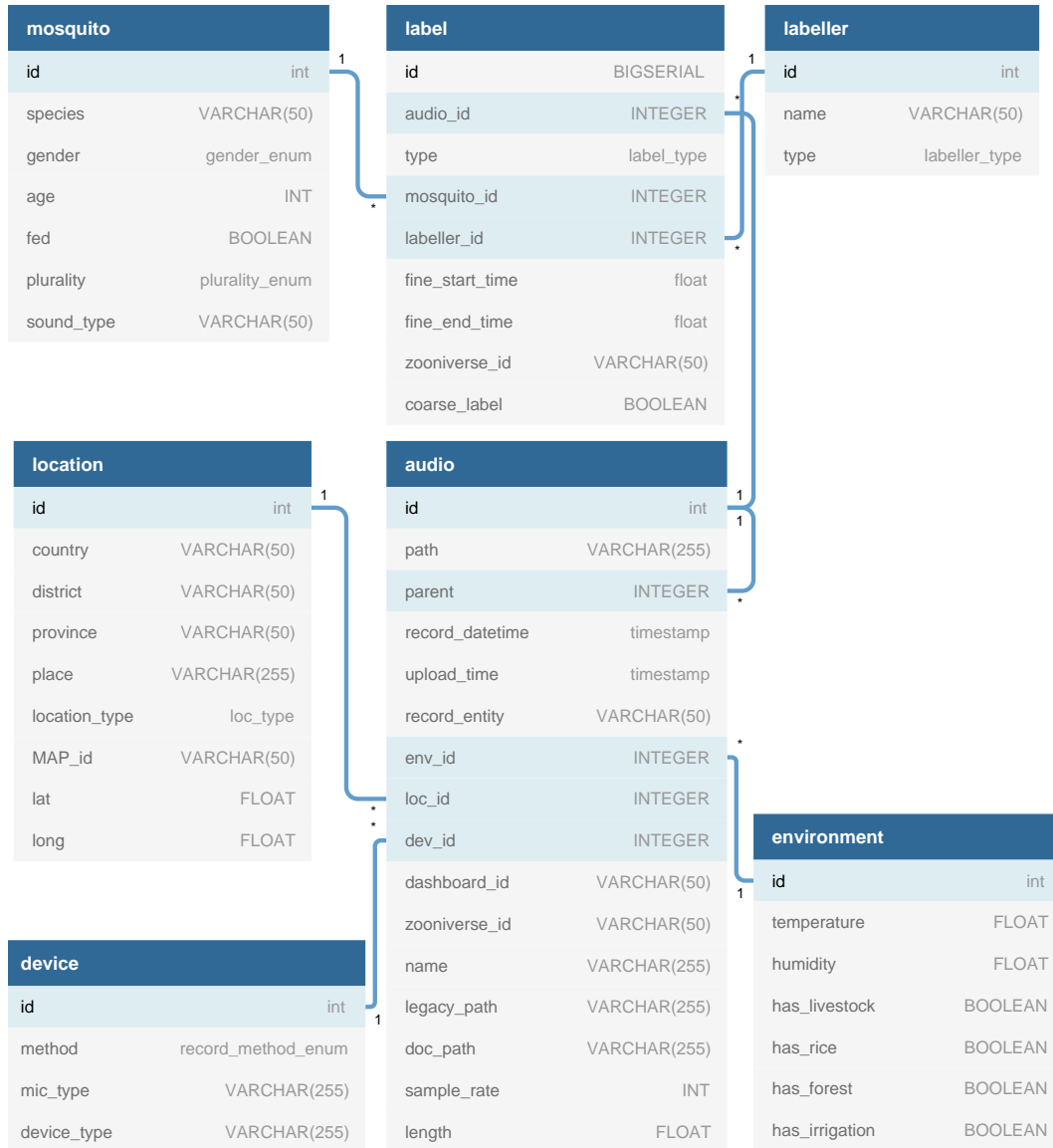
Figure 10: Relational tables of the full PostgreSQL database which was used to generate the data for this paper. The structured nature of the database enforces a standard in label format, ensuring we can efficiently mix and match data from a wide range of experiments with differing protocols. For example, if we wish to investigate the effect of mosquito gender or microphone type on the ability to detect mosquitoes, we may sub-select data with the appropriate metadata with one query. Database schema generated with dbdiagram.io from with pg_dump -s .
