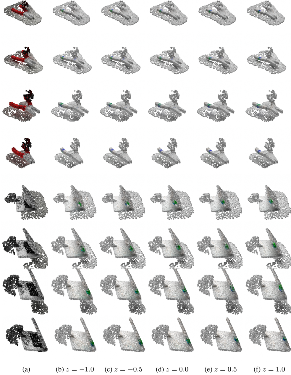
Figure 4: Visualization of sampled and generated 3D probability maps for the second grasp after the first grasp. From left to right in each row: (a) the colored 3D point cloud at the current manipulation state; (b)-(f) generated probability map of the next grasp given specific latent code z , where green and blue denote the finger 1 and 2 of the second gripper in the second grasping step. Zoom in for better a view of the figures.
