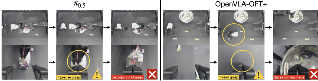
Figure 5: Common failure modes of \pi_{0.5} and OpenVLA-OFT+ on two challenging ALOHA robot tasks. Left: \pi_{0.5} struggles to execute a high-precision grasp and loses grip of the ziploc bag. Right: OpenVLA-OFT+ reaches between two candies rather than towards one, suggesting difficulty with modeling the highly multimodal action distribution.
