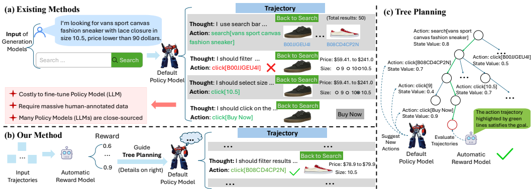
Figure 1: In Fig. 1 (a), we show that it is difficult for LLM agents to generate multi-step plans in an interactive environment to achieve the instruction goal. However, it is relatively easy for an LLM to learn a reward model that can evaluate whether the trajectories meet the task instructions, as shown in Fig. 1 (b). In Fig. 1 (c), we show that a learned reward model can be used to guide the default policy models to improve action planning.
