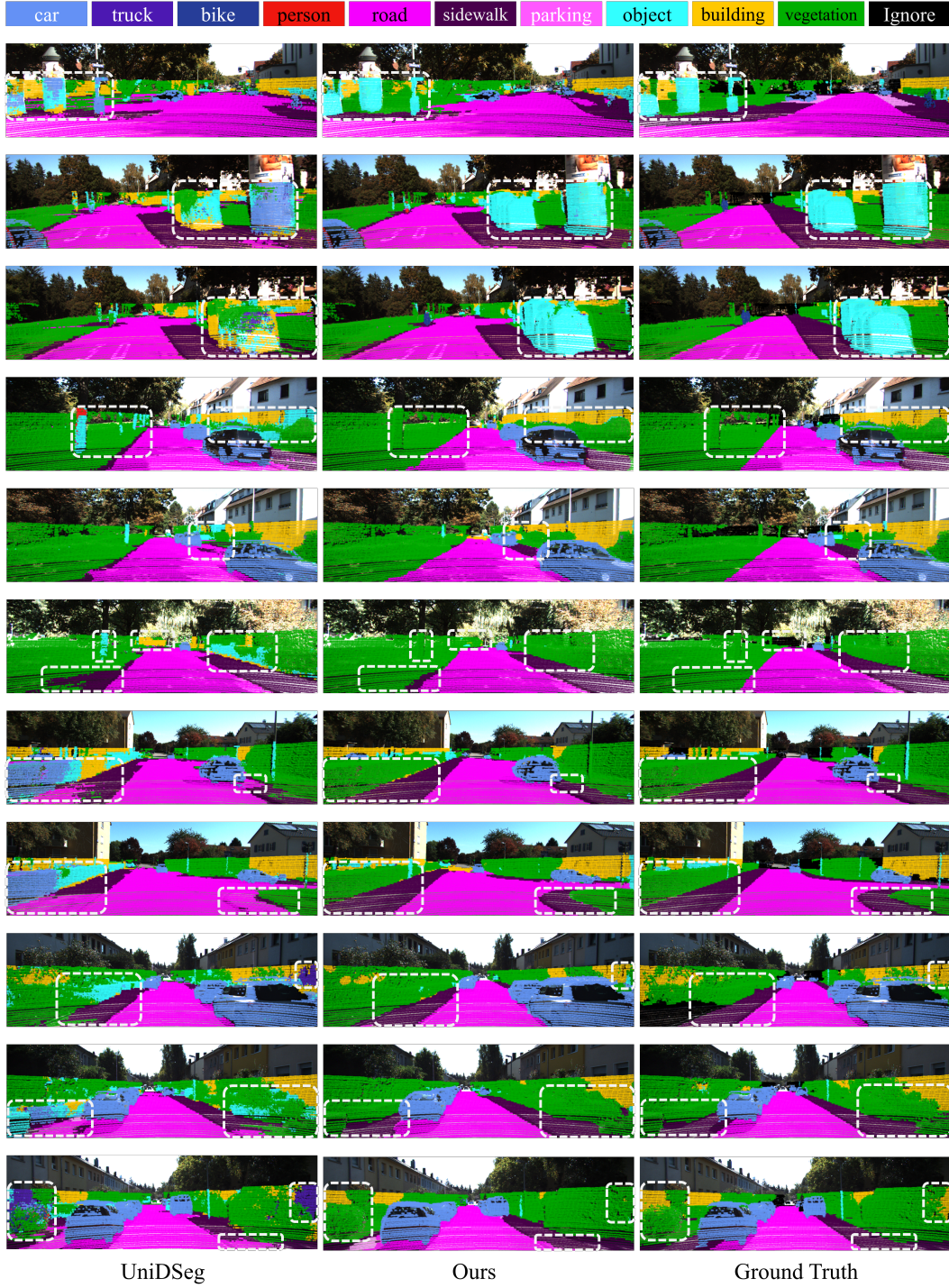
Figure 2: Qualitative results on A2D2→SemanticKITTI. From left to right: the visual results predicted by UniDSeg, Ours, and Ground Truth. We deploy the white dash boxes to highlight different prediction parts.
