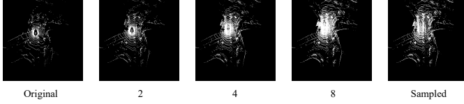
Figure 1: Integrate point clouds from different numbers of adjacent frames and finally perform random sampling on the merged point clouds. 2,4,8 denotes the number of adjacent frames being merged.
