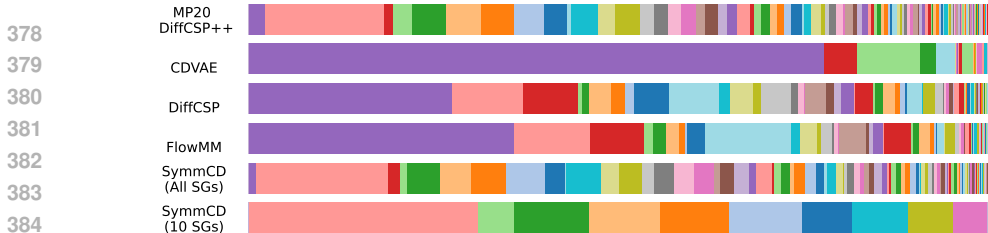
Figure 4: Proportion of space group symmetries of the dataset, and each method. The width of each color segment represents the proportion of crystals with that symmetry. From left to right, the first few space groups are: P1, Fm \bar{3} m, Cm, P \bar{1} , C2/m, I4/mmm, Pm \bar{3} m, P6 _3 /mmc, and Pm.
