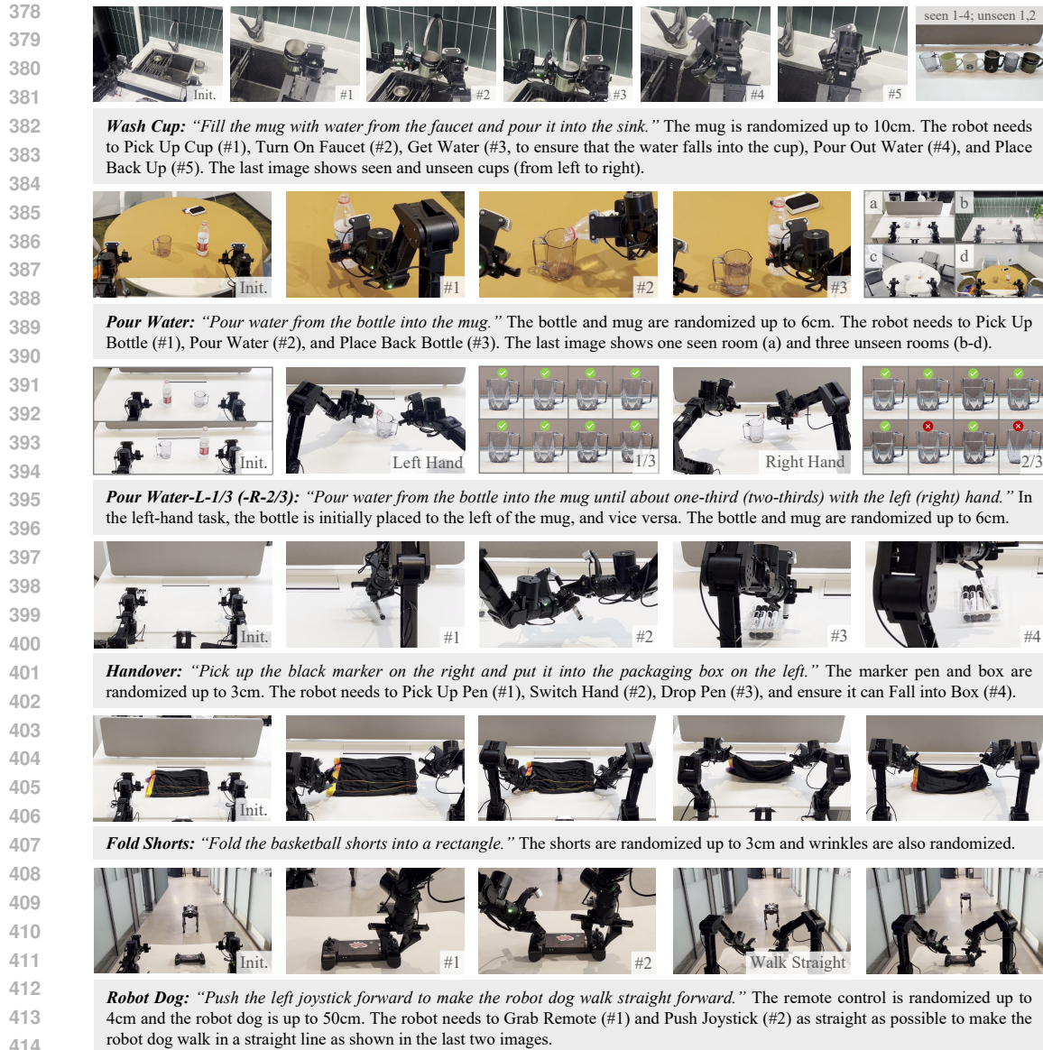
Figure 5: Task definitions and visualizations. For 7 challenging tasks, we describe their language instruction, randomization, and definitions of each sub-task. For Pour Water-L/13 and Pour Water-R-2/3 , we show the resulting water levels in two images.
