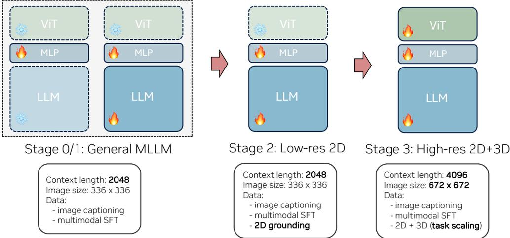
Figure 8: **Cube-LLM training pipeline.** We illustrate different stages of **CUBE-LLM** training pipeline. Stage 0 and 1 follow common MLLM training following (Liu et al., 2023a), Stage 1 trains 2D parts of LV3D in low-resolution with the vision encoder frozen. Finally, we fully finetune on all 2D and 3D parts of LV3D in high-resolution ( $672 \times 672$ ). In Figure 5 (bottom right, second) we compare this setup to combining the Stage 2 and 3 together.
