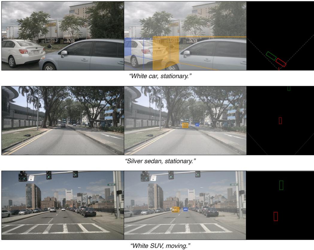
Figure 19: **Failure cases of DriveLM-Grounding images.** The error mainly attributes to semantic mismatch. Each row has the original image (left), projected 3D box prediction and ground truth (middle), and BEV image (right). **Blue box** is the ground truth and **Orange box** is the prediction. In BEV images, **Green box** is the ground truth and red box is the prediction.
