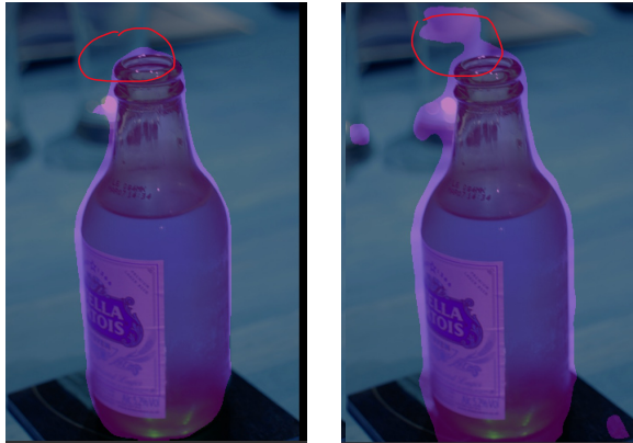
Figure 1: left :maxpooling right: avgpooling
